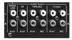
If your stereo doesn't have auxiliary inputs, you can also connect to any other pair of inputs; if you use the tape inputs, however, connect to the "play" jacks, not the "record" jacks. Once you're hooked up, set your stereo to play from whichever input you plugged into; most home stereo receivers have a dial or switch that toggles the input source (see Figure 3-4).
