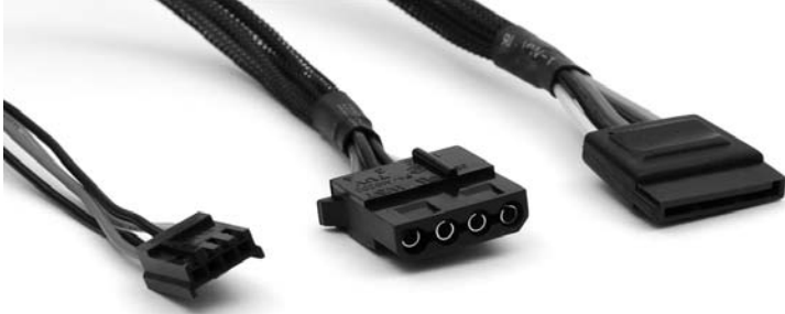
FIGURE 4.11 Mini, Molex, and SATA power connectors (left to right)
