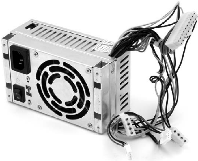
FIGURE 4.10 Proprietary power supply
