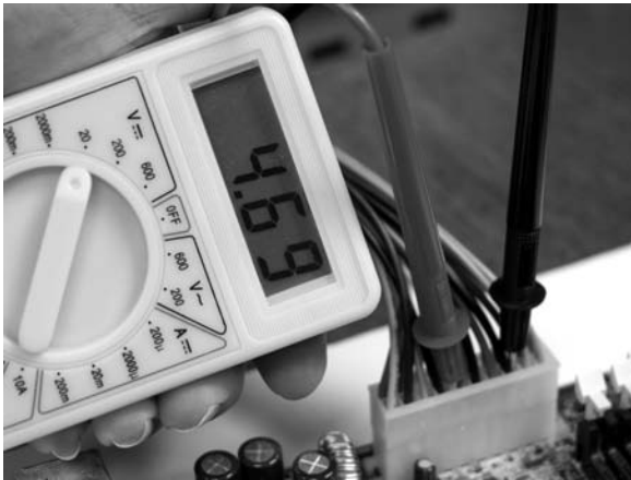
FIGURE 4.14 Testing one of the 5-volt DC connections
