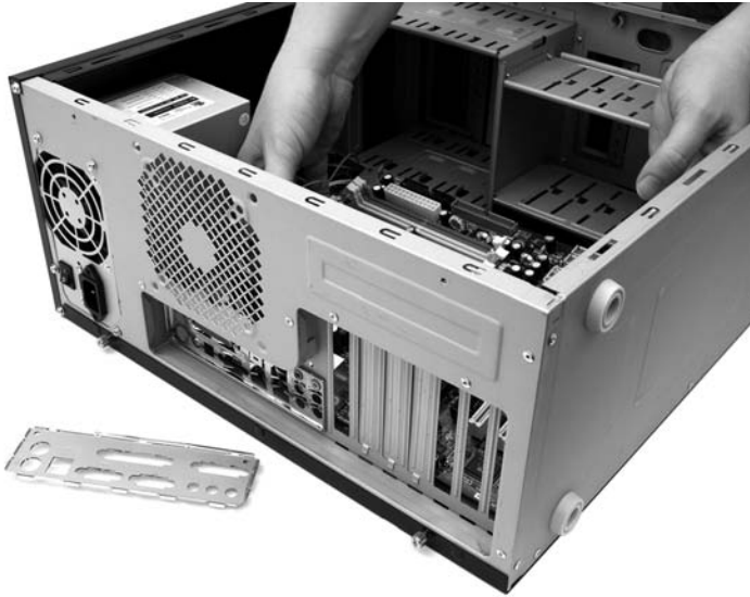
FIGURE 4.8 Installing a motherboard (note spare I/O shield)
