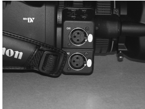
FIGURE 1-25 XLR microphone inputs (female)
