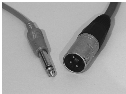
FIGURE 1-15 1/4" phone plug and XLR plug (male)
