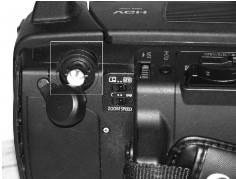
FIGURE 1-24 BNC connector (female)
