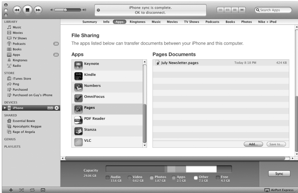
FIGURE 14-1 The File Sharing area on the Apps tab in the iTunes control screen for an iPhone lists the apps that can transfer files. Click an app to see its files.
