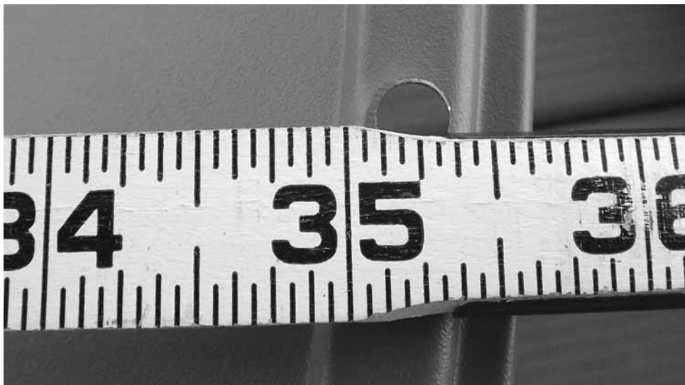
FIGURE 4-5 Horizontal axis measurement on 90 cm dish in inches
