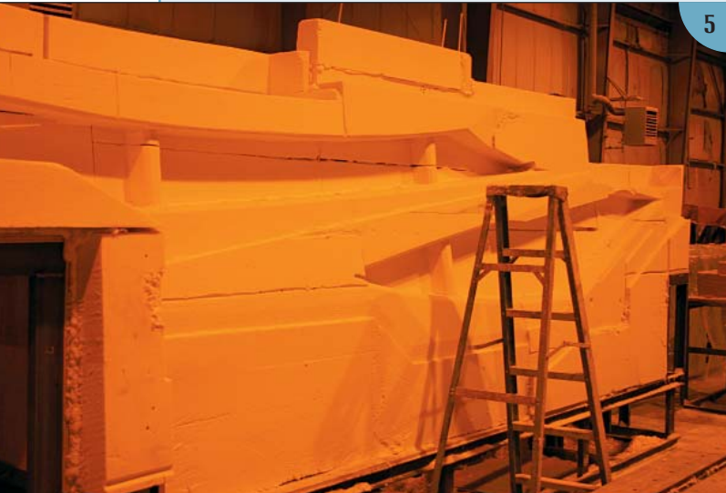
(5, 6, 7) The router at the D. L. Blount Associates production facility in Norfolk, Virginia, runs for two shifts a day to keep up with the workload. These parts for a large fiberglass yacht show some of the complex shapes that can be molded with a computer-controlled router. Note how the steps in photo 6 are cut into the bulkhead. (Courtesy D. L. Blount Associates)
