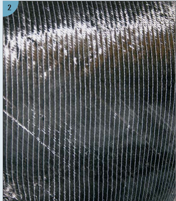
(2) A laminate of fiberglass and polyester resin has a tensile strength of about 27,000 psi (pounds per square inch), whereas a laminate of carbon fiber and epoxy resin has a tensile strength of about 61,500 psi.
