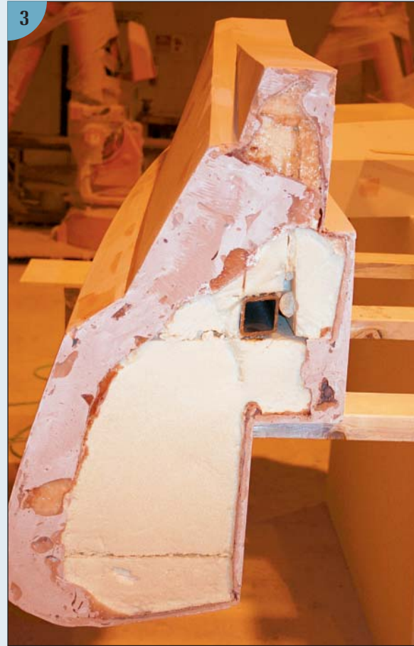
(3) Here you can see the parts of the finished plug. The steel armature is in the middle of the yellow foam section made of foam blocks. Pink fairing compound covers the layer of sprayed-on foam, but a little of it shows as a darker yellow than the foam blocks. This sprayed-on foam is cut by the five-axis router, and the fairing compound is applied over the newly cut surface. The router then goes back over the job to make a finish cut, which then receives a final handfairing.
