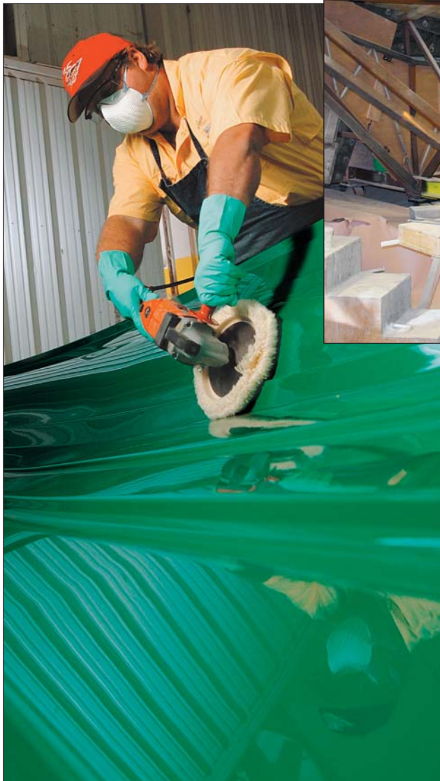
Multiple coats of mold release wax are applied to a hull mold and buffed out, creating a highly polished surface for laminating the hull. (Courtesy Ranger Boats)
