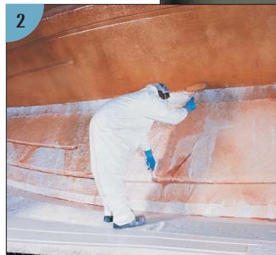
(1) Spraying gelcoat into a mold to form the polished exterior surface of a hull. (2) Rolling resin over fiberglass. (Courtesy Ranger Boats)
