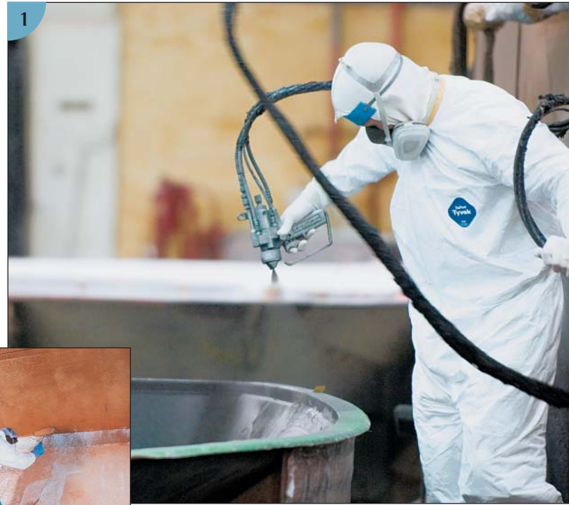
(1) Spraying gelcoat into a mold to form the polished exterior surface of a hull. (2) Rolling resin over fiberglass. (Courtesy Ranger Boats)
