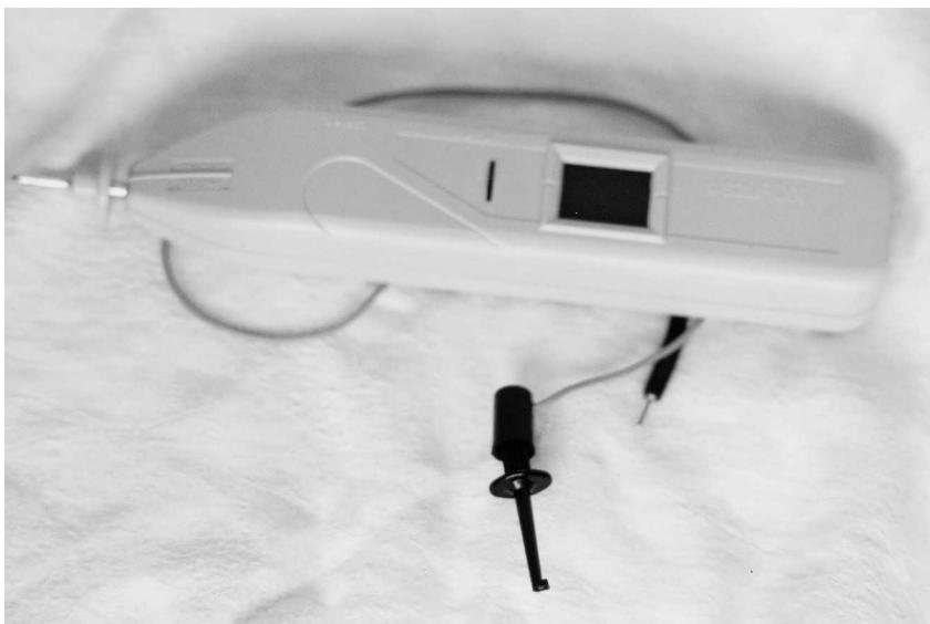
**Figure 215** OsziFOX hand-held digital oscilloscope
