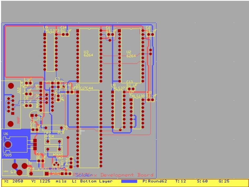
**Figure 197** Prototyping: putting power-control signals onto the PC board
