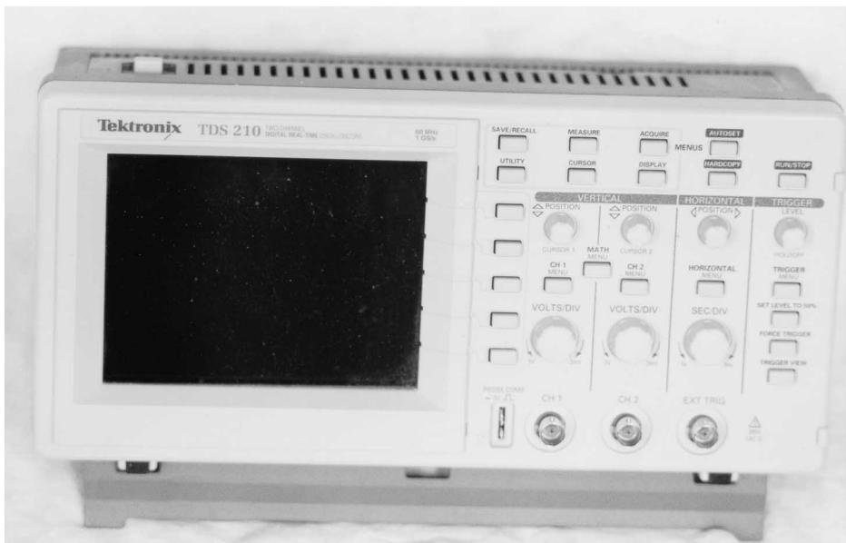
**Figure 211** TDS-210 digital oscilloscope
